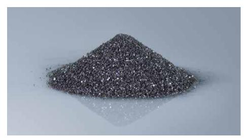
In the copper production process oxygen is a disruptive factor. It enters the melt and reacts with the copper to Cu<sub>2</sub>O. If it is not removed, it causes porosity of the casting. As a deoxidant, calcium hexaboride removes the detrimental copper oxide.
